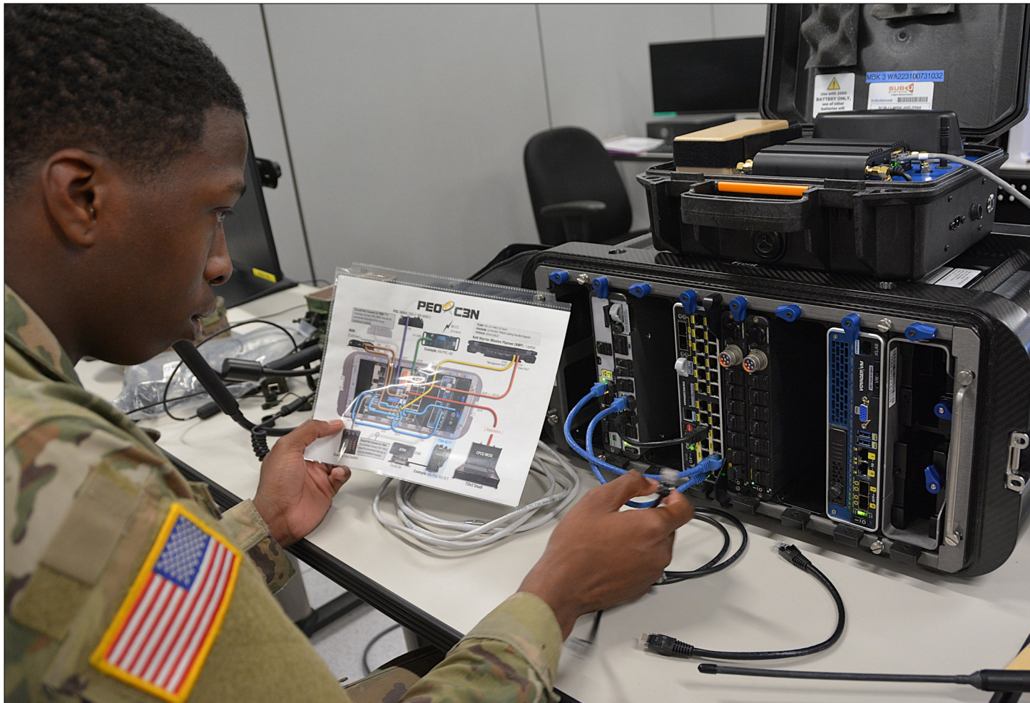
Sgt. Tyler Davis assembles a Tactical Radio Integration Kit as part of the Signal Digital Master Gunner course at Fort Gordon, March 18. Davis is a network communication systems specialist (25H) assigned to 442nd Signal Battalion, 15th Signal Brigade. (Photo by Laura Levering, U.S. Army Signal School)
