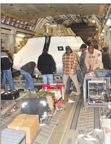
The mock Orion space capsule is prepared prior to a developmental test of the Capsule Parachute Assembly System (CPAS) on Dec. 20, 2012. The CPAS was rigorously evaluated at YPG in multiple developmental tests between 2011 and 2018. (Photo by Mark Schauer)
