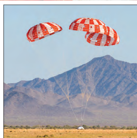
ABOVE: Test personnel examine components of the Orion Space Capsule's Capsule Parachute Assembly System (CPAS) after a test at U.S. Army Yuma Proving Ground (YPG) on July 18, 2012. The system was rigorously evaluated at YPG in multiple developmental tests between 2011 and 2018. LEFT: A mock Orion space capsule decelerated by the Capsule Parachute Assembly System touches down after a test at U.S. Army Yuma Proving Ground on September 13, 2018. (Photos by Mark Schauer)
