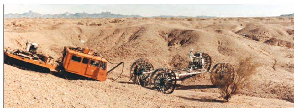
In 1966, the Mobility Test Article, an early version of the lunar rover, went through developmental testing on U.S. Army Yuma Proving Ground's vast ranges. The final product traversed the moon in 1971 and 1972. (US Army photo)
