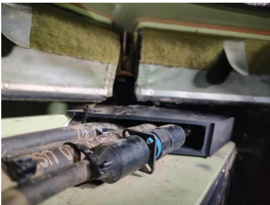
Figure 6. Image of CAN bus cables with 3D printed bracket installed. (Image by SFC Donald Fadel)
