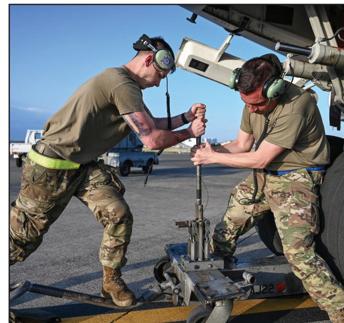
(left) Senior Airman Marcus Simones, left, 445th Aircraft Maintenance Squadron aerospace maintenance technician, and Master Sgt. John McDermott, 445th MXS jet mechanic, use a tire jack on nose landing gear to replace tires on a C-17 Globemaster III at Yokota Air Base, Japan, April 14, 2025. (Photo by Tech. Sgt. Johnathan Quinones) (right) A fire truck and three pallets of humanitarian goods are loaded onto a 445th Airlift Wing C-17 Globemaster III at Wright-Patterson Air Force Base, May 8, 2025, for transport to Belize. (Courtesy photo)
