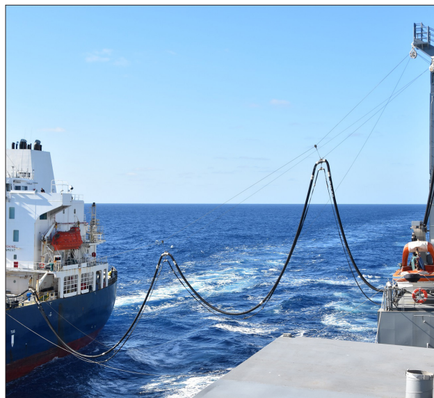
Military Sealift Command's (MSC) dry cargo ammunition ship USNS Matthew Perry (T-AKE 9) connects fuel lines with MSC chartered tanker MT Badlands Trader during a consolidated cargo replenishment operation in the vicinity of Okinawa, Japan, Dec. 15. (U.S. Navy courtesy photo)
