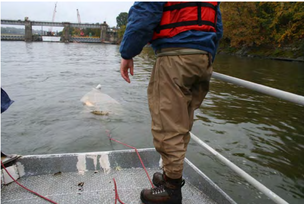
Figure 4. Collecting surface waters with the meter nets. Meter nets contain a flow meter mounted inside the net to determine the volume of water passing through and are used to capture fishes swimming on or near the surface.
