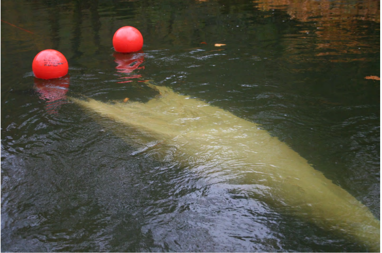
Figure 5. Suspending the surface trawl with floats. The benthic trawl has been modified to allow electrified sampling of fishes swimming on or near the surface.
