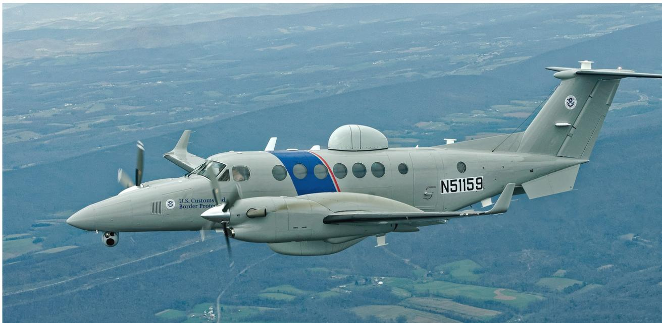
The Multi-Role Enforcement Super King Air 350ER (MEA) is a medium-range, fixed-wing, twin turboprop aircraft. It's used by U.S. Customs and Border Protection, Air and Marine Operations (AMO) to conduct aerial patrol and surveillance over land and water, and for enforcement relocation of personnel and equipment.
