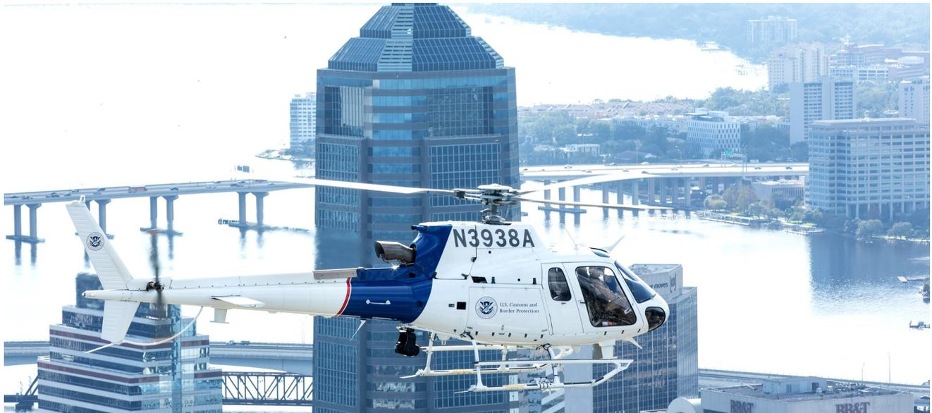
The Helicopter AS350/ H125 Light Enforcement Helicopter (LEH) is a short-range, turbine-powered helicopter used by U.S. Customs and Border Protection, Air and Marine Operations to perform missions such as aerial patrol and surveillance of stationary or moving targets. These LEHs are the optimal aerial surveillance platform in metropolitan areas because their vertical lift capability and maneuverability enable operations from off-airport sites and within close proximity to congested airports.
