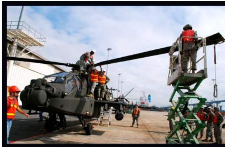
(Above) Soldiers from TF Falcon work to fold blades of Apaches deploying with the brigade to Afghanistan, Oct. 6 at the Georgia Port Authority's Ocean Terminal
