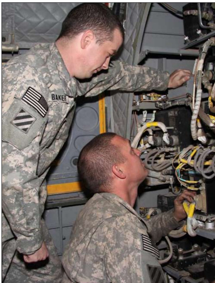
(Top) Spc. Robert Dubose of D Co., TF Knighthawk, inspects the hydraulic deck of a Black Hawk for corrosion during a corrosion control inspection, Feb. 20 at Bagram Airfield. (Bottom Left) Sgt. John Baker and Spc. Matthew Lopez of D Co., TF Knighthawk, are reinstalling radios in the avionics closet of a Chinook during a 400-hour phase inspection, Feb. 20, at Bagram Airfield. (Bottom Right) Staff Sgt. Michael Ortiz (left), briefs Capt. Travis Betz, both D Co., TF Knighthawk, on the maintenance progress that has been made, Feb. 24 at Bagram Airfield.
