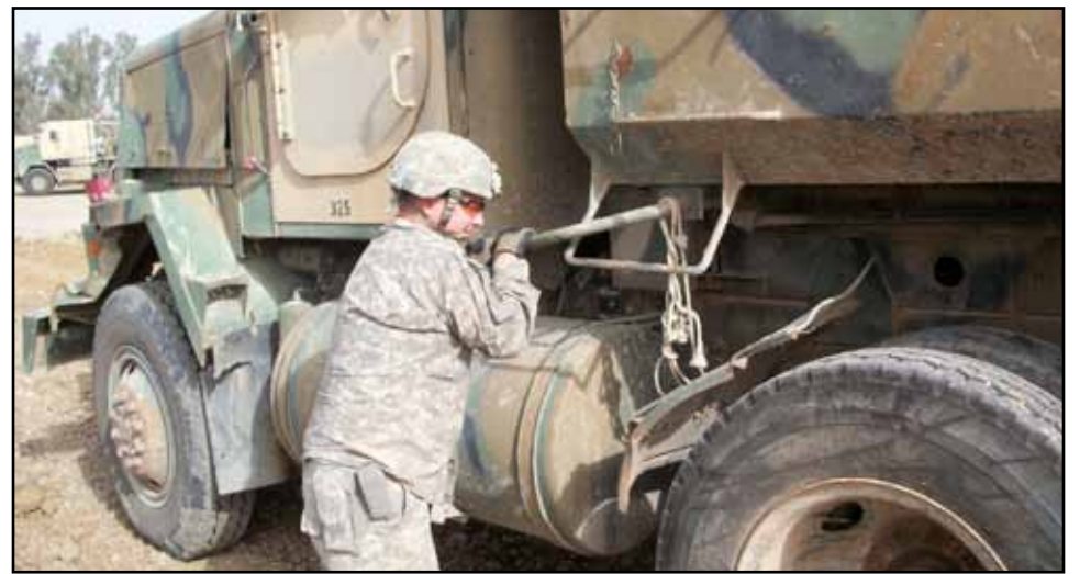
Staff Sgt. Jason Clark, 317th Engineer Company, prepares a 20-ton dump truck to empty a load of gravel. Two dump trucks brought dirt and gravel to fill in low spots in the Mobile Redistribution Team's yard. The added material should improve the yard greatly, bringing an end to the flooding when it rains.
