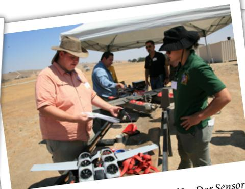
JIFX 21-4 participant Stuart Dana of SpyDar Sensors Inc. holds one of six motors used in their electric ducted fan propelled unmanned aerial vehicles. The Vertical Take-Off and Landing prototype and its larger cousin were demonstrated at the quarterly field experiment site, Aug. 24. (U.S. Navy photo by Javier Chagoya)
