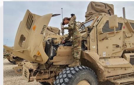
SPC Canales conducting PMCS on an MRAP that the Service Members use to conduct security checks.
