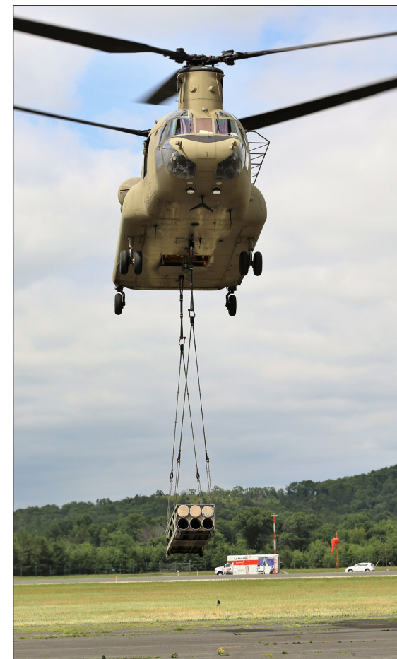
A Chinook helicopter lifts the connected load June 27 after the loading team has safely moved to an area outside the loading zone.
