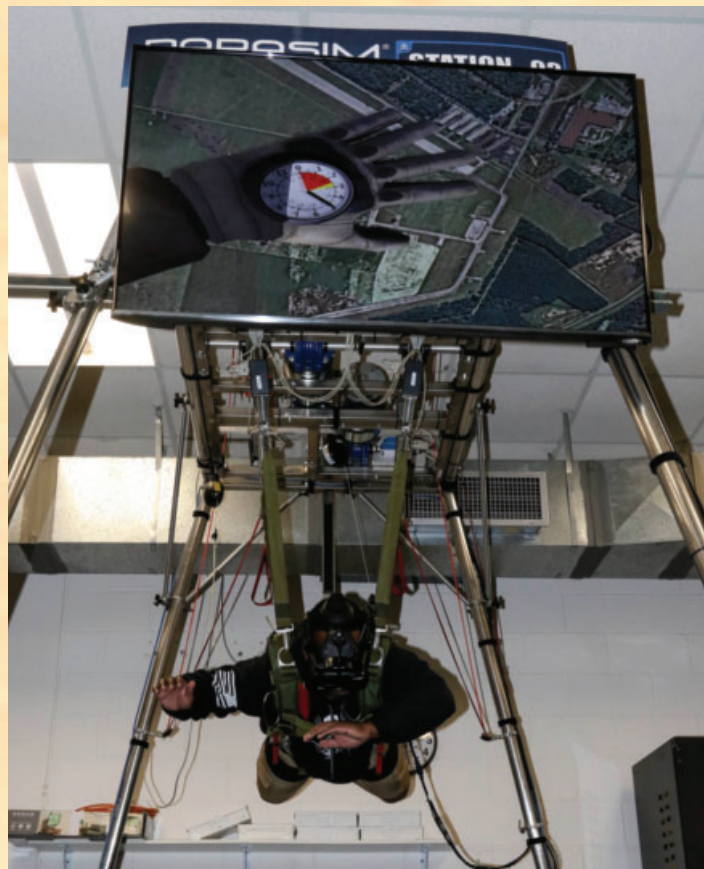
A paratrooper participates in a virtual reality jump training on the new Parachute Simulator 7 at the Joint Riggers Facility, MacDill Air Force Base, Tampa, Fla., Feb. 21. Photo by U.S. Army Staff Sgt. Stephen M. Colvin.
