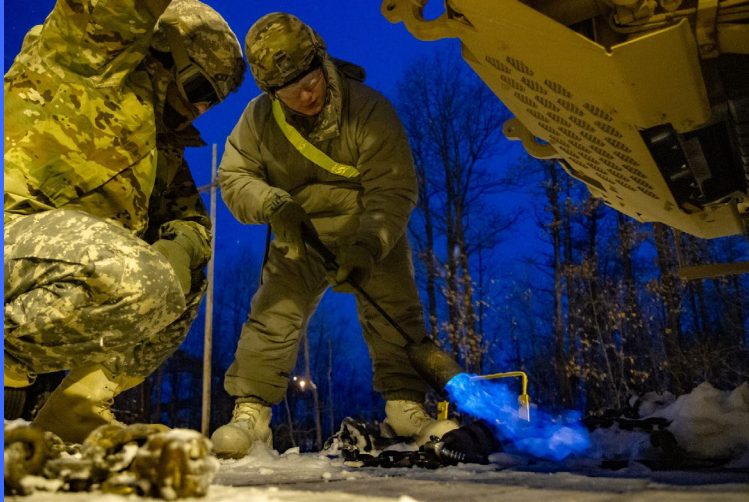
Pvt. Ryan Trumm uses a blowtorch to de-ice vehicle tie-down chains during railhead operations in preparation for JRTC, Jan 23, 2019, Fort Drum, N.Y.
