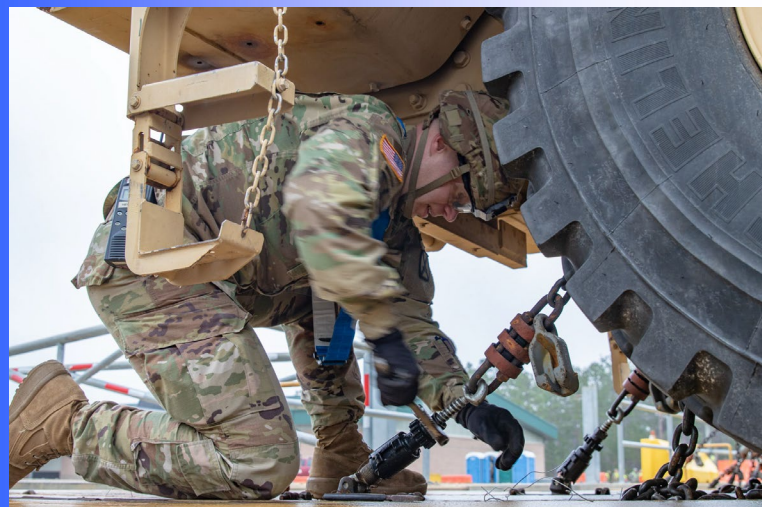
Maj. Etheridge, Executive Officer, 2-22IN, loosens a tie-down chain from a M977 HEMTT (Heavy Expanded Mobility Tactical Truck) on a cargo train during the 1BCT, 10MTNDIV, training rotation at the Joint Readiness Training Center, Fort Polk, La., Friday, Feb 1, 2019.
