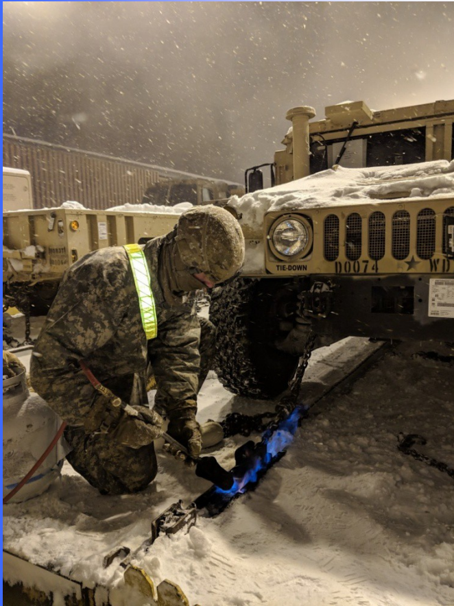
A Soldier from 1BCT uses a torch to melt the ice build up on a chain that connects the vehicle to the railhead car, Jan 28, 2019.
