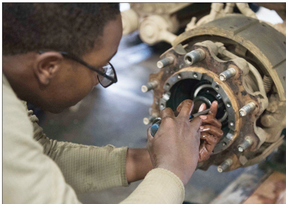
Pfc. Deshawn Presswood, a 135th Forward Support Company, 188th Brigade Support Battalion, light wheel vehicle mechanic, takes out a bearing from a M142 HIMARS.
