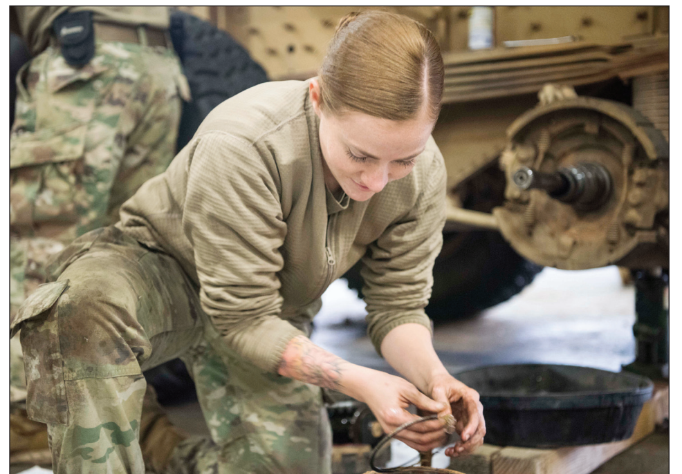
Spc. Savannah Padilla, a 135th Forward Support Company, 188th Brigade Support Battalion multiple launch rocket system repair mechanic, takes out a seal on a wheel hub of a M142 HIMARS.
