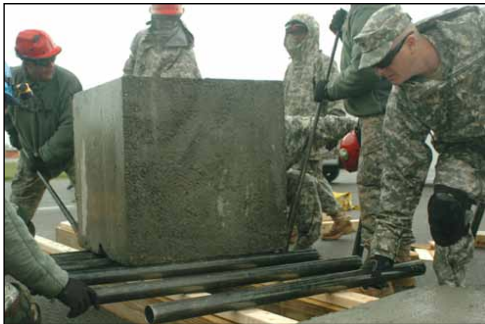
ORISKANY, N.Y. – Sgt. John Grace, a Long Beach, N.Y. resident and member of the 1156th Engineers Company’s Search and Extraction Team, places a roller in front of a two-ton block as it moves 75-feet past obstacles at the New York State Preparedness Center May 14. (U.S. Army Photo by Spc. J.p. Lawrence, 42nd Inf. Div. PAO).
