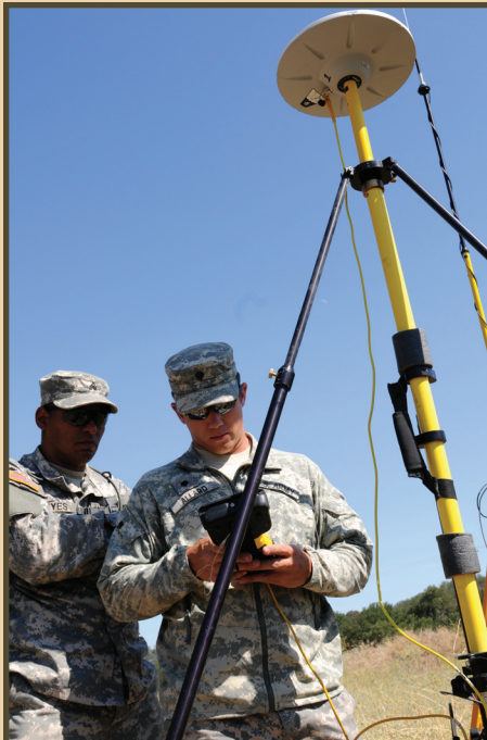
Spc Benjamin Allard, 372nd Engineer Brigade calibrates the global positioning system on the base while Sgt. Vinicio Reyes, 605th Engineer Detachment looks on at Fort Hunter Liggett, Calif. Aug 4. The base is calibrated with two rovers to acquire precise topographical elevation measurements. (Photo by Sgt. Francis Horton, 363rd Public Affairs Detachment)
