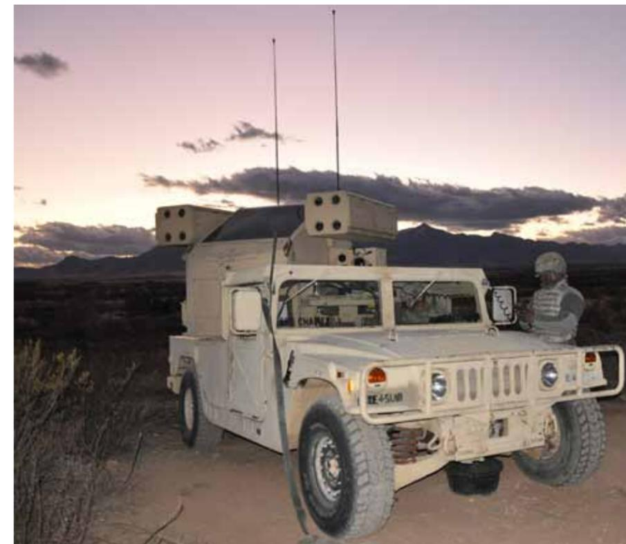
Pfc. Ronnie Thompson, an Air and Missile Defense crewmember, conducts a systems check of an Avenger weapon system. The Avenger system was used in conjunction with Sentinel radars to detect aircraft attempting to illegally enter U.S. airspace along the U.S. – Mexico border in Arizona.
