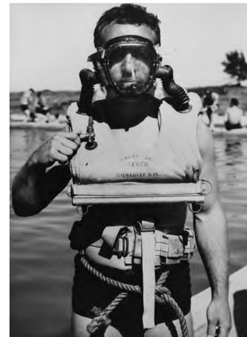
An underwater demolition team diver demonstrating early Navy SCUBA gear with full face mask in 1944.
