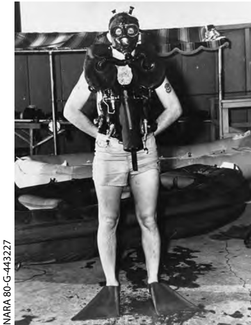
An underwater demolition team diver demonstrating a Lambertson rebreather unit at a National Research Council Symposium in 1951.
