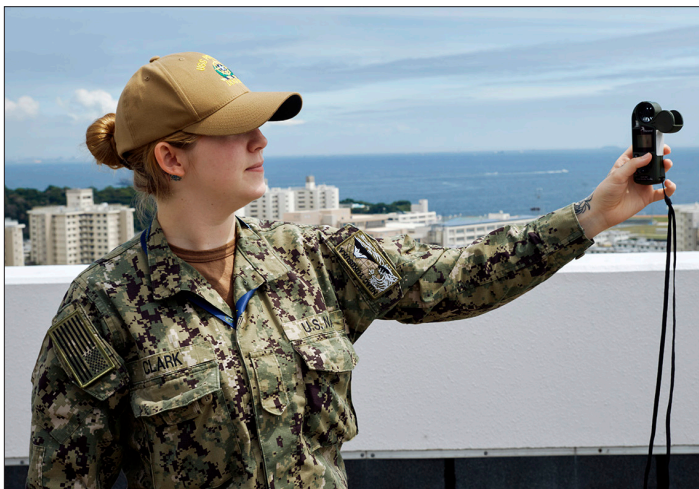
Airman Sara Clark of Naval Oceanography Anti-Submarine Warfare Center (NOAC) Yokosuka demonstrates the Kestrel May 27, 2026. The Kestrel is a rugged, handheld weather meter and environmental data logger designed to measure and track specific atmospheric conditions including wind speed and direction, temperature, pressure, and altitude, among other data points. The NOAC Yokosuka team tracks the weather to protect Fleet Activities Yokosuka Sailors, military families, and the places they live and work while serving as a critical resource for asset protection and risk management for Commander, U.S. Naval Forces Japan/Region Japan (CNFJ/RJ) ashore forces and U.S. 7th Fleet afloat personnel and ships. (Photo by James Kimber, CFAY Public Affairs)
