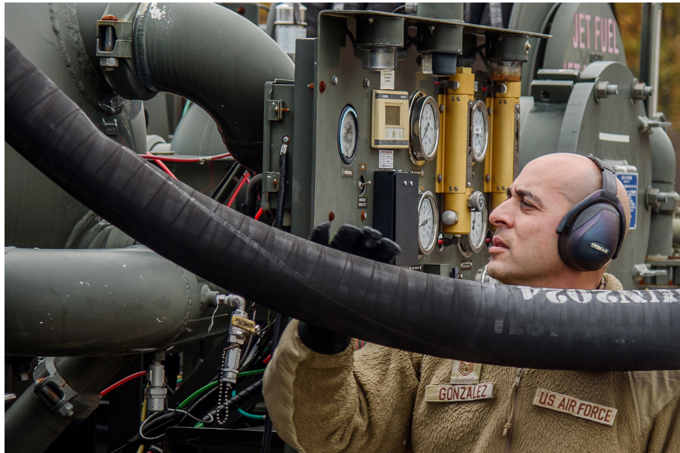
U.S. Air Force Airmen with the 108th Logistics Readiness Squadron perform weekly and monthly maintenance checks on an R-12 Hydrant Servicing Vehicle to prevent potential maintenance issues and ensure that proper refueling mission can take place. The R-12, which connects directly to the in-ground piping system can refuel up to 1,000 gallons per minute.
