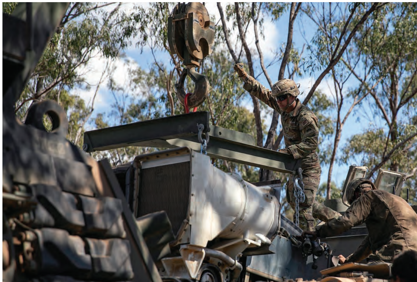
SGT Caelib Gustafson, an M1A2 Abrams tank mechanic assigned to Comanche Company, 4th Battalion, 6th Infantry Regiment, helps guide the crane operator as they lower an engine into the body of an M1A2 Abrams tank at the Townsville Field Training Area, Townsville, Australia, Aug. 9, 2023. (Photo by SPC Charlie Duke)
