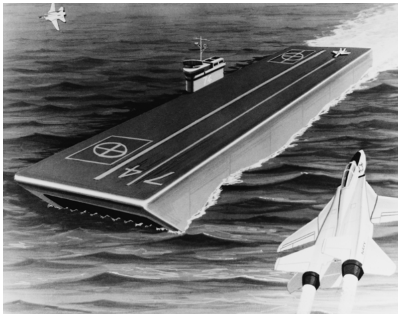
Artist's conception of an aircraft carrier version of the proposed high-length-to-beam surface effect ship type, February 1976. (NHHC, USN 1165638)
