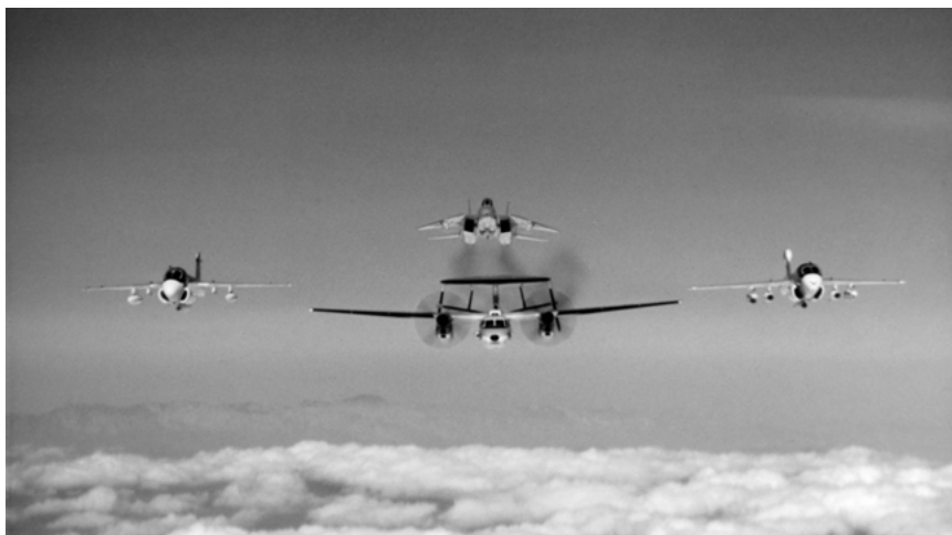
A Grumman E-2C “Hawkeye” AEW aircraft leads a group of other Grumman- aircraft in formation. At top is an F-14 Tomcat fighter. An A-6E Intruder attack plane is at left , and an EA-6B Prowler electronic warfare plane is at right . The teaming of the Hawkeye with the Tomcat was fundamental to Navy air defense in the 1970s and 1980s. (NARA, K-116900)
