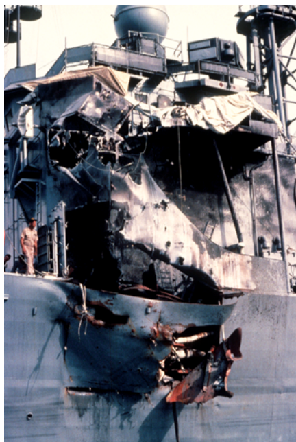
External damage to the port side of Stark from the two Iraqi Exocet hits and the ensuing fire. (NARA, 6443167)
