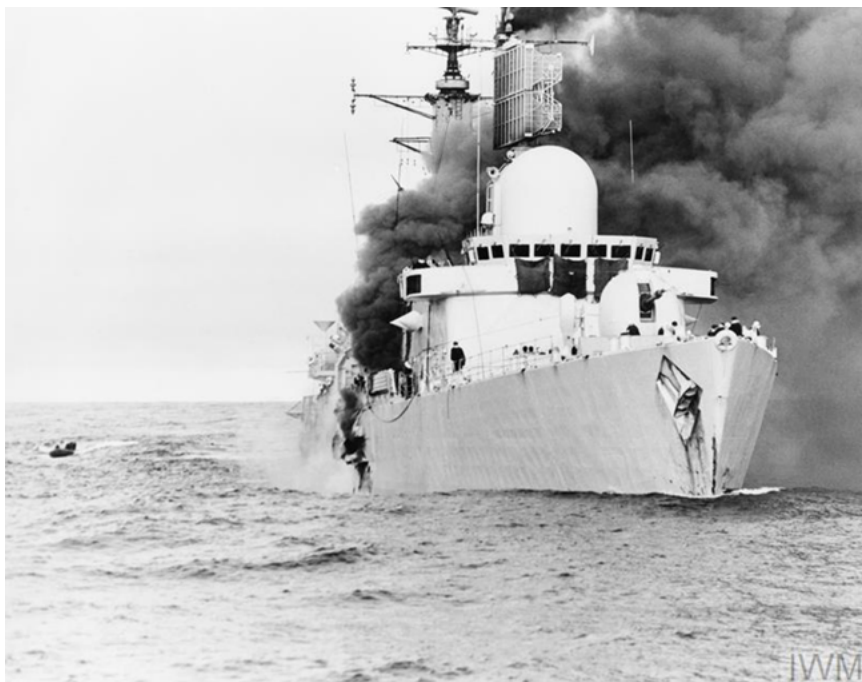
The Type 42 destroyer HMS Sheffield on fire after being struck by an AM-39 Exocet missile fired by an Argentine Super Etendard on 4 May 1982. The hole in the ship's starboard side is clearly visible. (Crown copyright reproduced under delegated authority from The Keeper of Public Records. Image: Imperial War Museum FKD 66)
