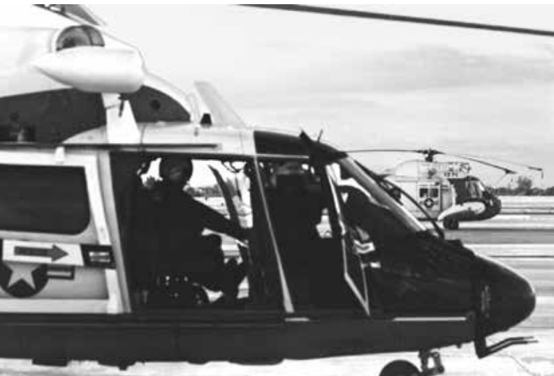
MIAMI – A Eurocopter HH-65A Dolphin sits on the ramp at the U.S. Coast Guard Air Station Miami with an older Sikorsky H-52 Seaguard amphibious helicopter parked in the background. The new Dolphins replaced the older Seaguards at Air Station Miami in 1985. U.S. Coast Guard photo.
