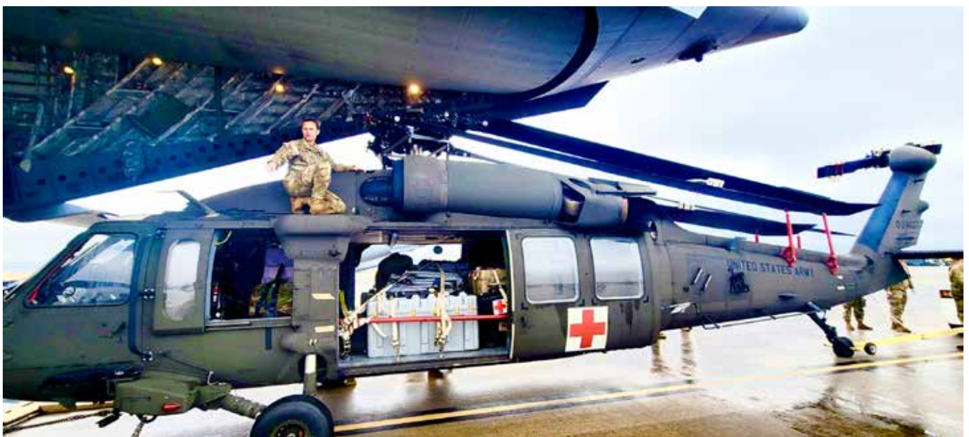
A UH-60 MEDEVAC being loaded onto a C-17 at the Charlotte National Guard AF ramp, North Carolina. Photo provided by the author.
