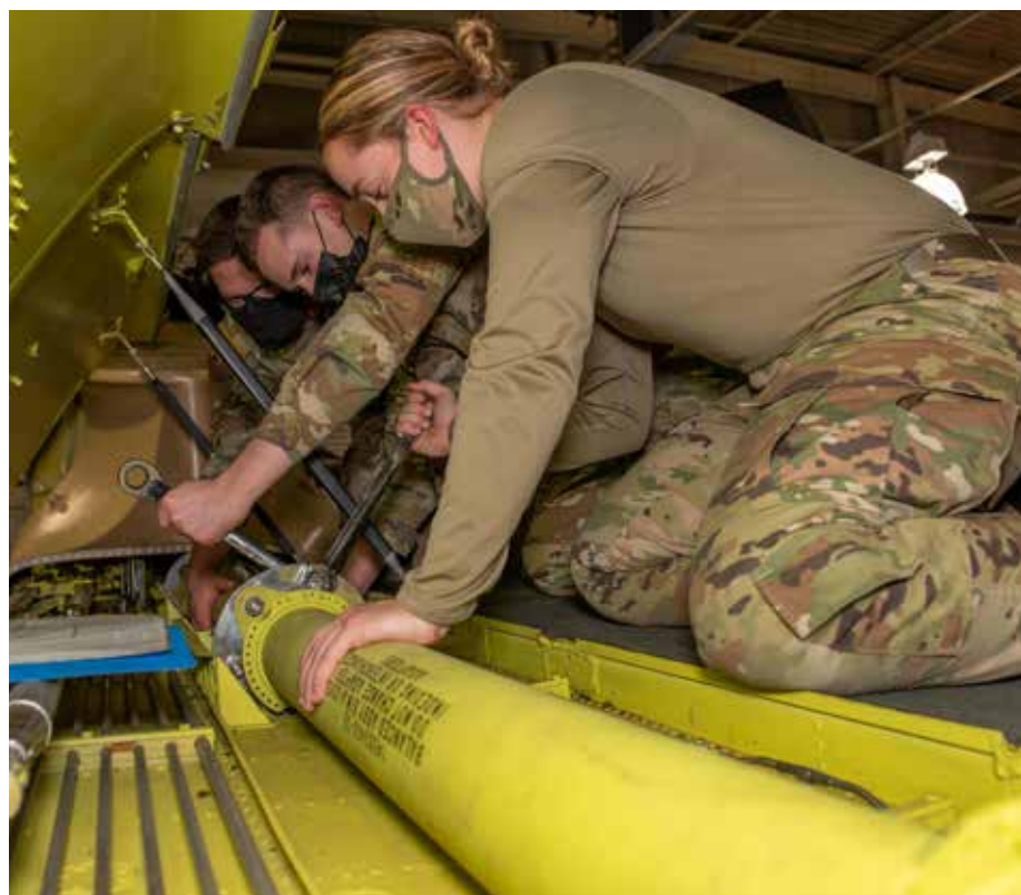
U.S. Army Soldiers installing torque tube bolts on a CH-47 training aid. After the 17-week Advanced Individual Training, they will become qualified MOS skill 15U, CH-47 Chinook helicopter repairers. U.S. Army photo by SSG George Prince.
