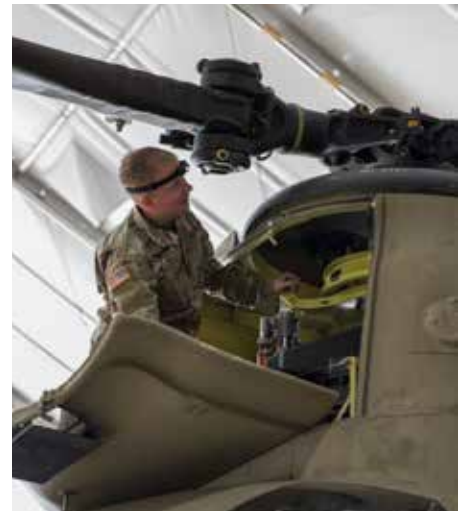
A CH-47 Helicopter Repairer (15U) works to replace a combining transmission (C-box) on a Chinook at a Fort Hood Airfield. U.S. Army photo by SGT Sydney Mariette.
