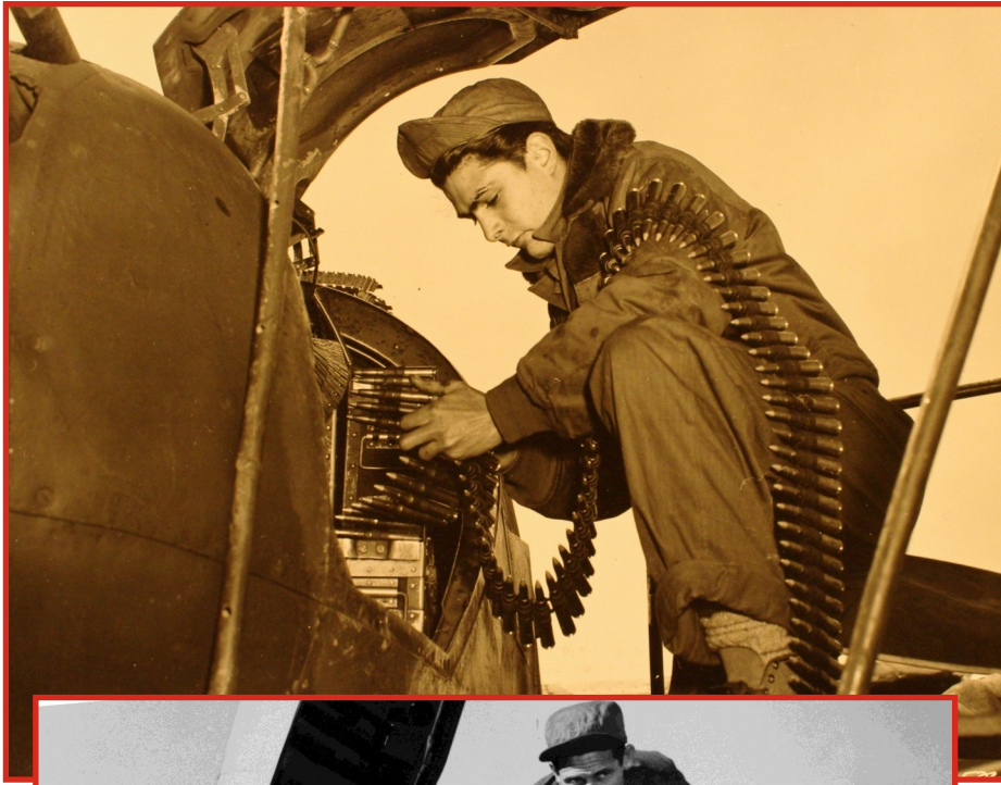
Left: Airman 1st Class Joseph J. Plezpert, Chicago, Ill., loads the nose guns of a U.S. Air Force B-26 light bomber with .50 caliber ammunition. An armament specialist, he loads the light bombers of the 3rd Wing with bombs, rockets, napalm and .50 caliber ammunition in preparation for the coming night's mission against the Communists. The night intruders strike against the enemy's warehouses, marshaling yards and troop concentrations. April 1952.
