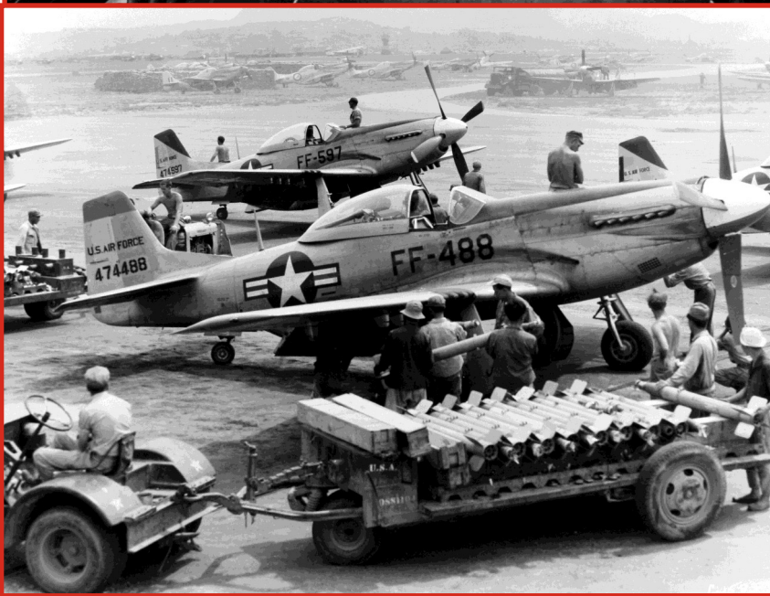
Above: When F-51 Mustangs of the Fifth Air Force's 18th Fighter Bomber Wing return from combat, they are met by skilled loading crews and mechanics to ready them for another immediate strike. Carts of 5-inch rockets and .50 caliber machine gun ammunition pull up, and armorers have the sturdy fighters ready for another in an average of seven minutes. July 1951.
