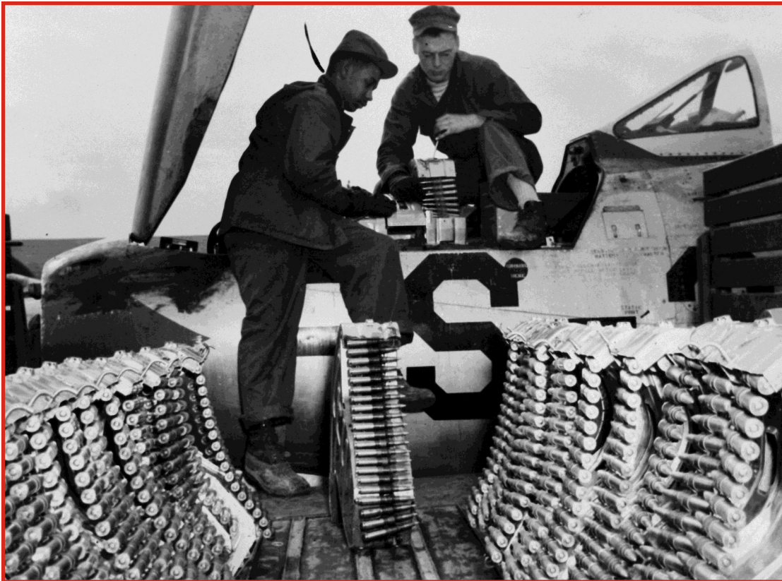
Above: Belts of .50 caliber machine gun ammunition are draped neatly into containers in the armament shops of the U.S. Far East Air Forces 27th Fighter Escort Group, loaded into trucks, and delivered directly to the F-84 Thunderjets which will deliver them to enemy Communist targets in Korea. By this efficient system, a small crew can service a large number of jet fighters in a remarkably short period of time. Loading a full container are Pfc. Fred O. Ferguson, Philadelphia, Pa., left and Pfc. Dwight W. Davis, Seattle, Washington, armament technicians of the 27th Group. 20 February 1951.
