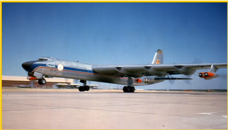
The Convair XB-36H 'Crusader' carried a nuclear reactor aboard the aircraft, though it never powered the bomber in flight. Convair photo.
