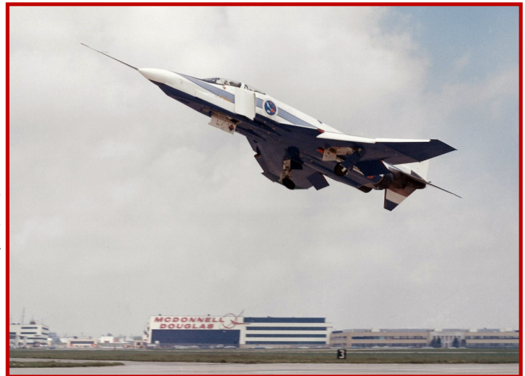
YF-4E #12200 takes-off from Lambert Field in St. Louis, MO, for the first flight of the Survivable Flight Control System (SFCS) program on 29 April 1972, to become the first fighter aircraft to use a fly-by-wire control system. (Mark Nankivil Collection)
