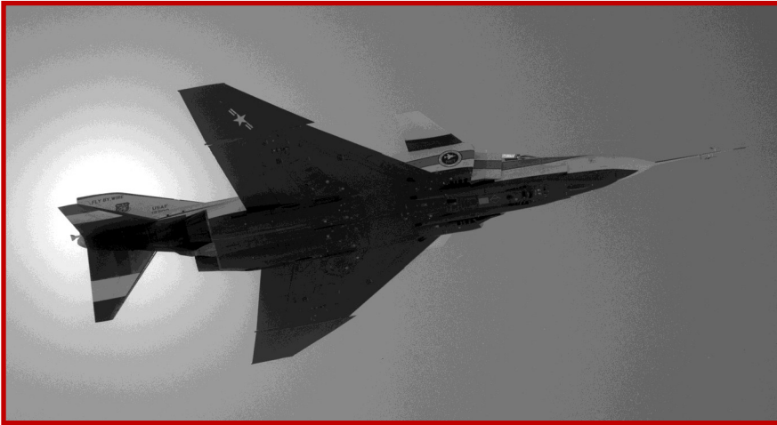
The dark blue bottom (FS 15044) and lack of wing leading edge slats show up well in these 2 inflight views of the YF-4E over Edwards AFB on 12 August 1974 at left. (USAF Photos by Sgt. Wayne Berry-AFTC History Office Collection)
