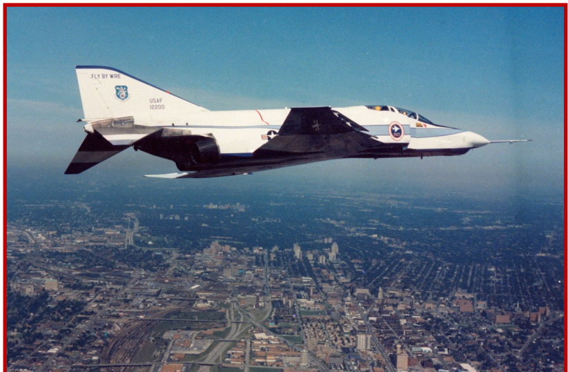
The canards mounted on the shoulders of each intake have a span of 5 feet with a surface area of 17 square feet. The outer 3 feet of each canard is removeable and a single test flight was accomplished utilizing the partial-span canards. (USAF Illustrations)
