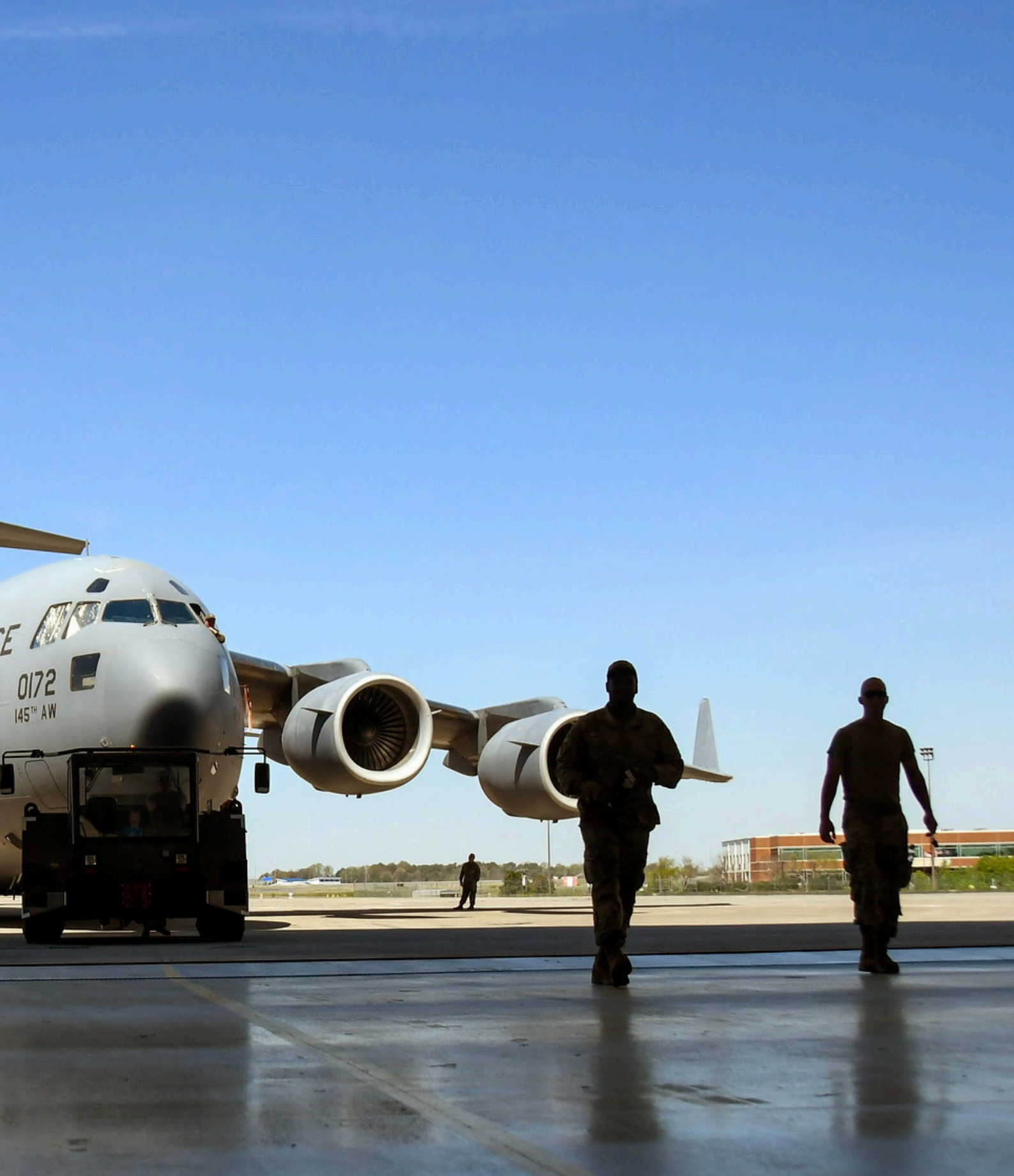
U.S. Air Force maintainers from the 145th Aircraft Maintenance Squadron tow a C-17 Globemaster III inside a hangar at the Charlotte-Douglas International Airport base, March 28, 2025. It takes 11 maintainers to safely tow the aircraft into the hangar with four engine stands. U.S. Air National Guard photo by 2nd Lt. Mary McKnight
