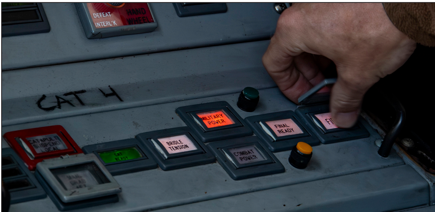
FIRE. The Integrated Catapult Control System (ICCS) or "bubble" is used to initiate a launch sequence.
