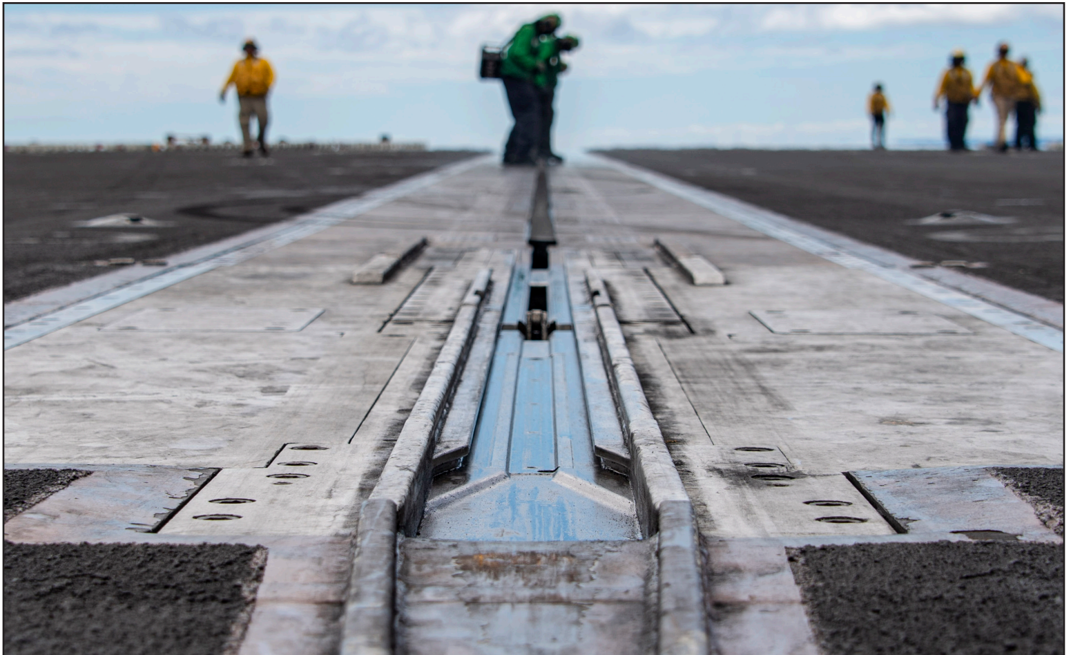
RUNWAY. Aircrafts are launched from zero to 165 knots, in less than two and a half seconds from these tracks.
