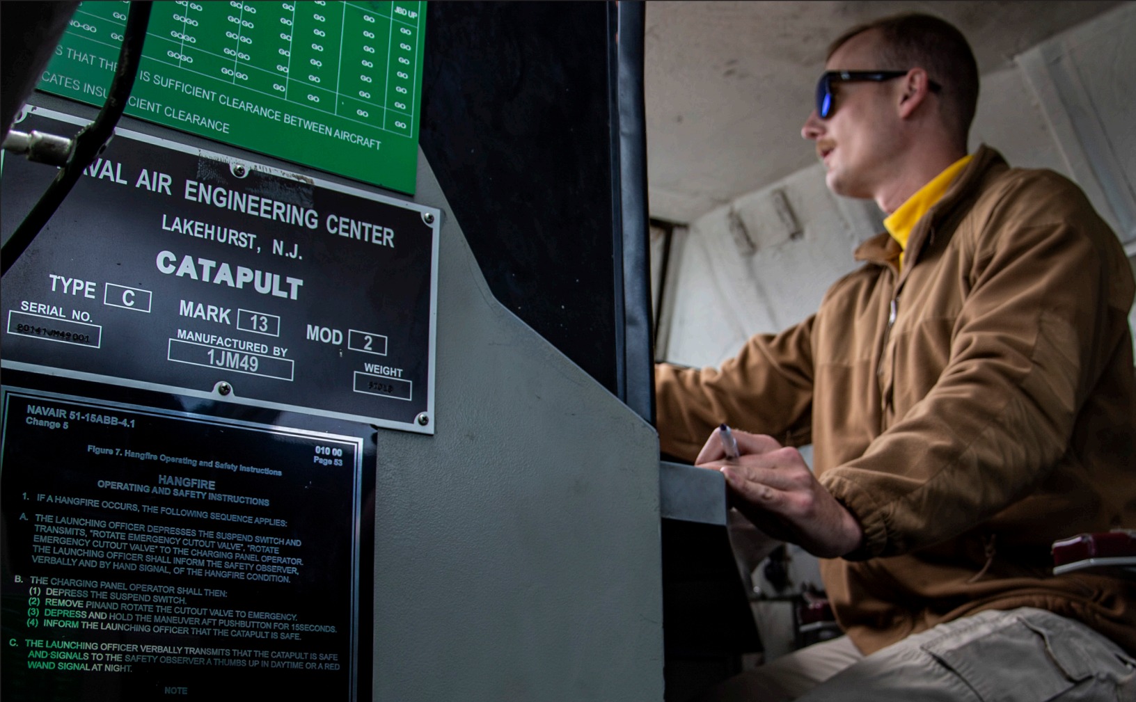
CONNECTION. The ICCS or "bubble" combines current remote stations to provide intercommunication during each aircraft launch.
