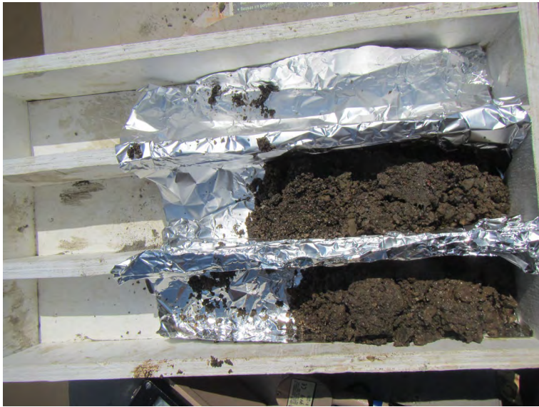
SVD-SD003, 2-6 feet (No 0-2 feet Recovery)
