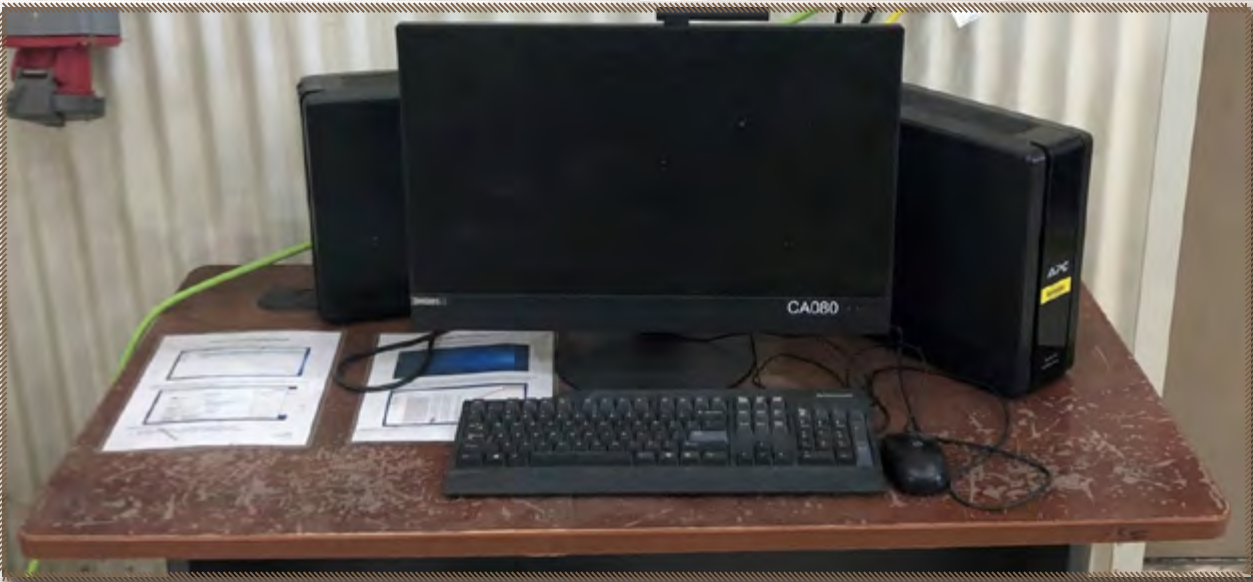
Standard Fort Novosel M1 SDS computer station setup in each shop. The computer has an uninterrupted power system (shown to the right) to ensure power stays on even during power outages. Laminated sheets provide a step-by-step guide on how to use the SDS tool. (Britt Dave)
