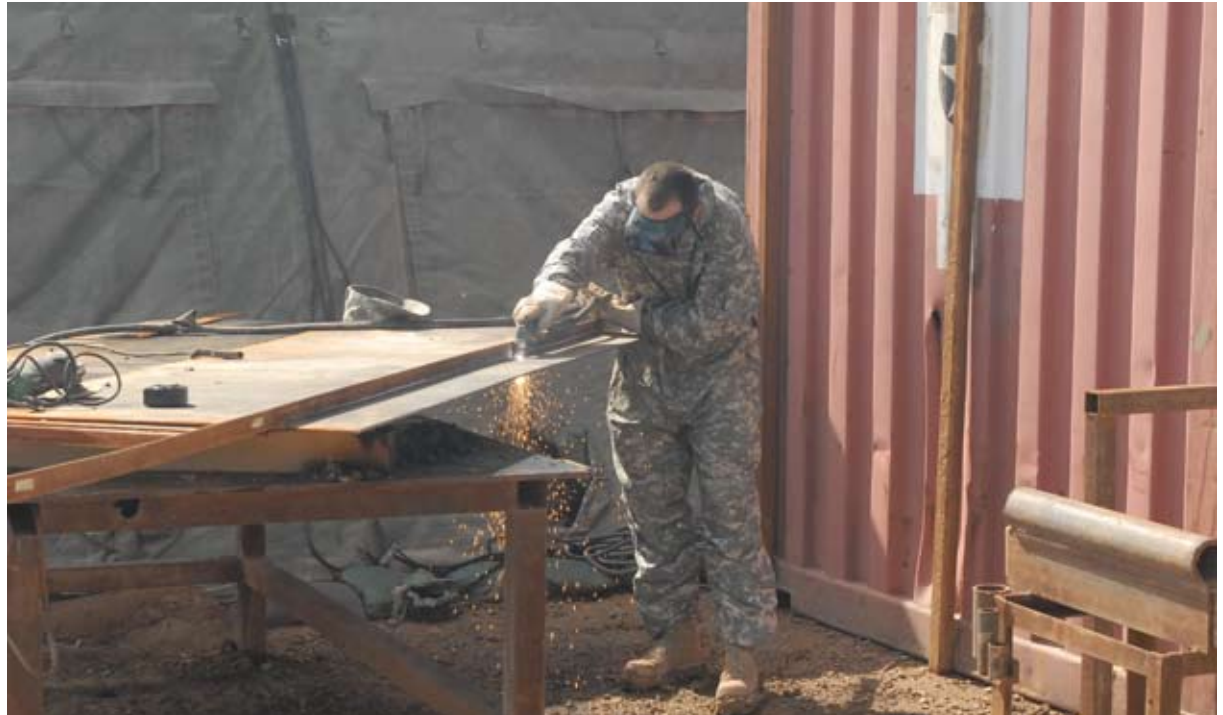
BAGHDAD — A Soldier from Company B, 210th Brigade Support Battalion, 2nd Brigade Combat Team, 10th Mountain Division's Monster Garage uses a plasma cutter to fabricate armor to be welded on to an Iraqi Federal Police Ford F350 from a sheet of metal at Contingency Operating Site Hammer March 1. Once completed, the truck will be delivered to the 1st Federal Police Division to better protect their personnel during patrols through their area of operations. (Army photo by Staff Sgt. Ryan Sabin, 2nd BCT Public Affairs)
