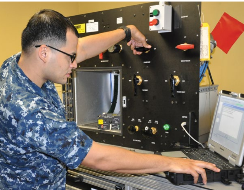
▲ Aircrew Survival Equipmentman 2nd Class Yithzack Licon tests crew oxygen regulators for a C-130 Hercules aircraft at Fleet Readiness Center Mid-Atlantic Detachment Washington. (U.S. Navy photo by Gary Younger)
