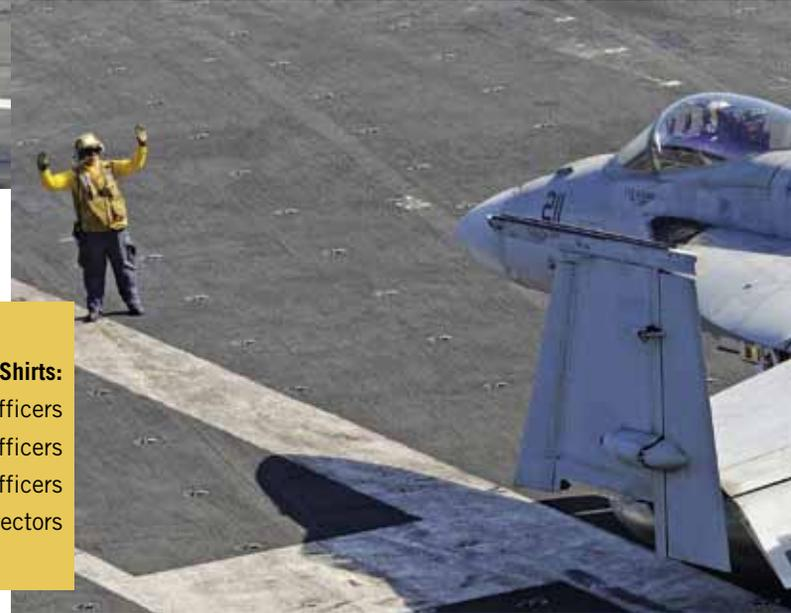
An aviation boatswain's mate guides an F/A-18E Super Hornet assigned to the Kestrels of Strike Fighter Squadron (VFA) 137 into launch position on the flight deck of the Nimitz-class aircraft carrier USS Abraham Lincoln (CVN 72). Photo by Mass Communication Specialist Seaman Zachary S. Welch.
