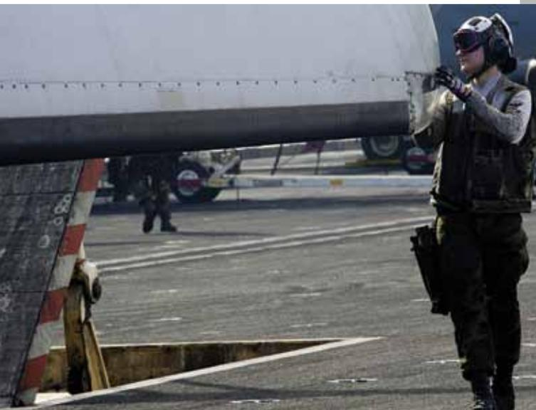
**Aviation Structural Mechanic 3rd Class Tia Squirres performs pre-flight checks on the wing of an E-2C Hawkeye from the Golden Hawks of Airborne Early Warning Squadron (VAW) 112 on the flight deck of the Nimitz-class aircraft carrier USS John C. Stennis (CVN 74). Photo by Mass Communication Specialist 3rd Class Kenneth Abbate.**
