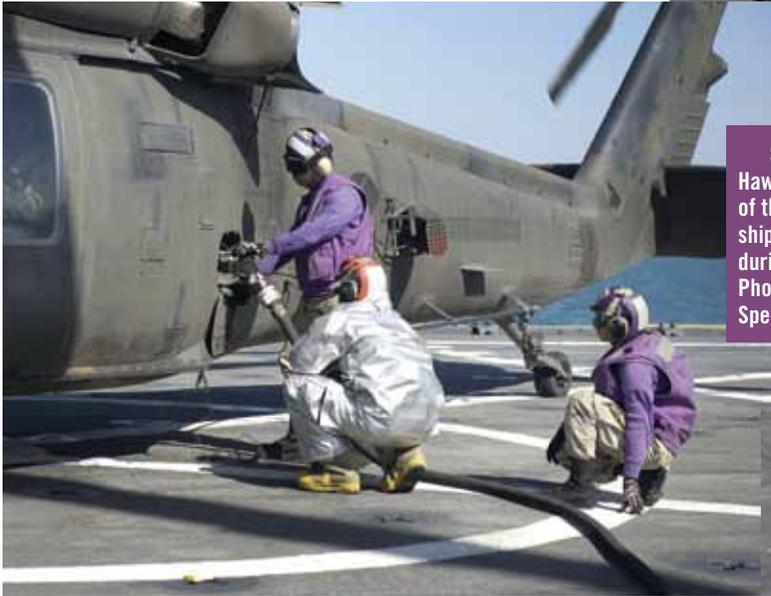
Sailors refuel an MH-60S Sea Hawk helicopter on the flight deck of the amphibious dock landing ship USS Pearl Harbor (LSD 52) during a deck landing qualification. Photo by Mass Communication Specialist 2nd Class Jason Behnke.
