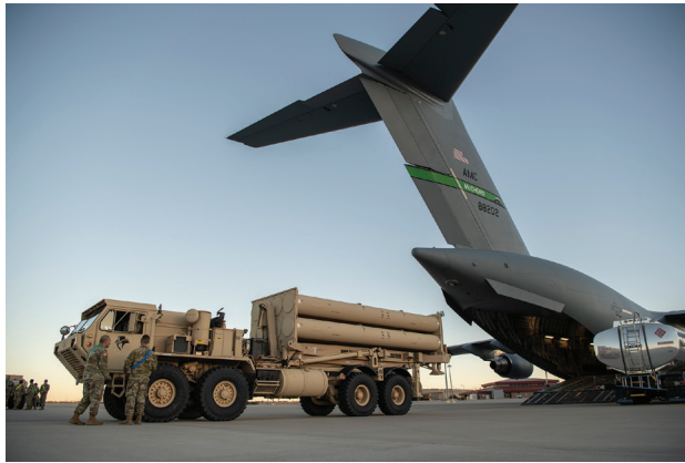
A U.S. Army Terminal High Altitude Area Defense launching station prepares to load onto a 4th Airlift Squadron C-17 Globemaster III at Fort Bliss, Texas, Feb. 23, 2019. The THAAD missile system is a land-based platform capable of intercepting ballistic missiles both inside and just outside the atmosphere. (U.S. Air Force photo by Staff Sgt. Cory D. Payne)
