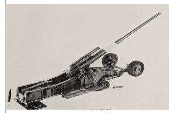
The T-145 175 mm Gun mounted on carriage T76E1. Shown is a model rendering of the gun which was developed directly from the M65 Atomic Cannon. The 175 mm Gun was one of three different mounts that was affixed to the triple threat carriage, along with the 203 mm howitzer and the 240 mm gun. The system was designed to be fielded in as little as four minutes.
