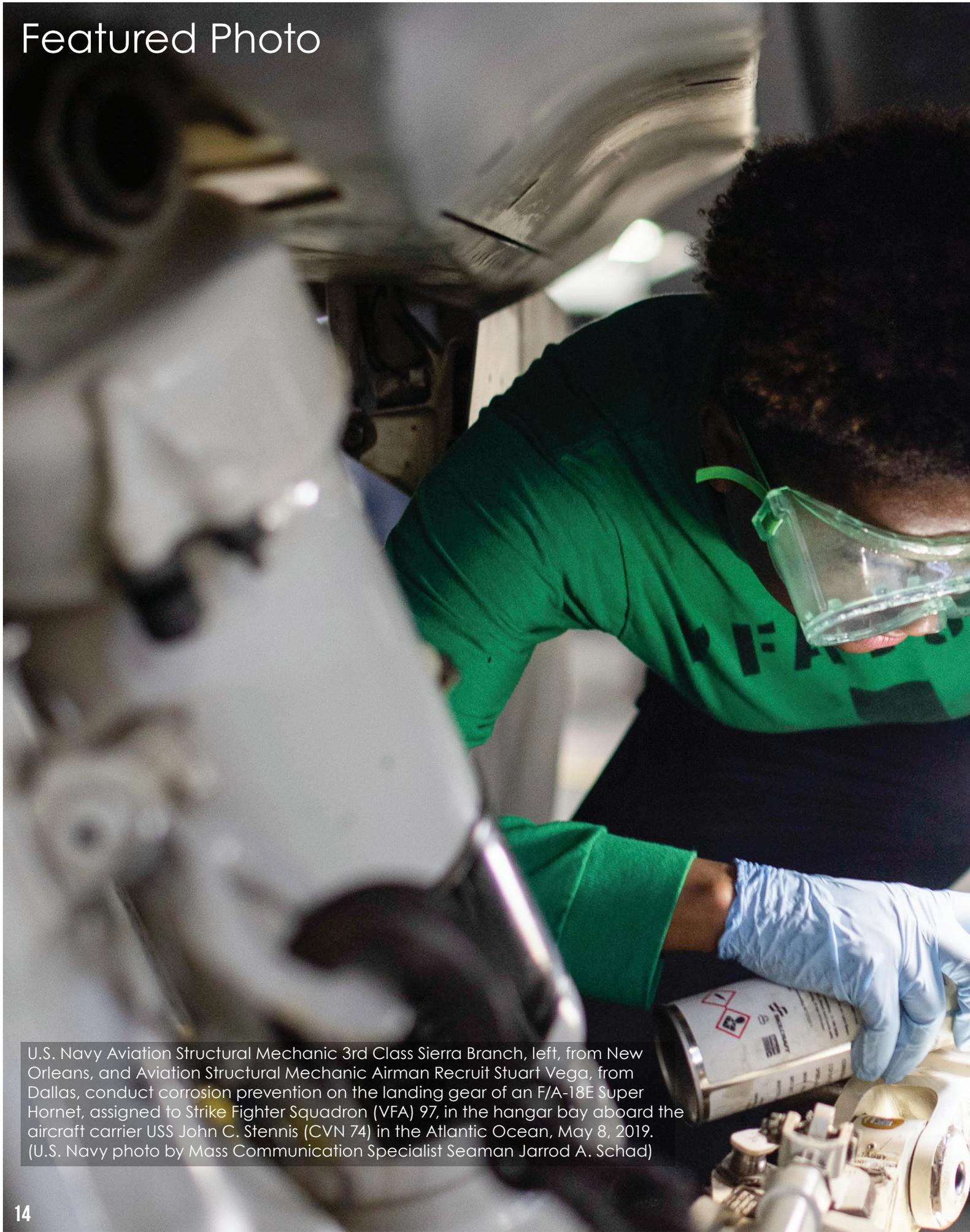
U.S. Navy Aviation Structural Mechanic 3rd Class Sierra Branch, left, from New Orleans, and Aviation Structural Mechanic Airman Recruit Stuart Vega, from Dallas, conduct corrosion prevention on the landing gear of an F/A-18E Super Hornet, assigned to Strike Fighter Squadron (VFA) 97, in the hangar bay aboard the aircraft carrier USS John C. Stennis (CVN 74) in the Atlantic Ocean, May 8, 2019. (U.S. Navy photo by Mass Communication Specialist Seaman Jarrod A. Schad)
