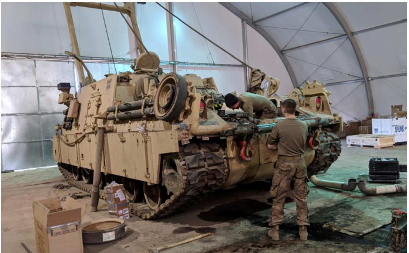
E Co, 101st BSB maintenance teams have been working diligently to repair all pacing items, to include the Battalion’s M88 Recovery Vehicle. The M88 is essential in ensuring all vehicles make it safely to training events in case of emergencies.
