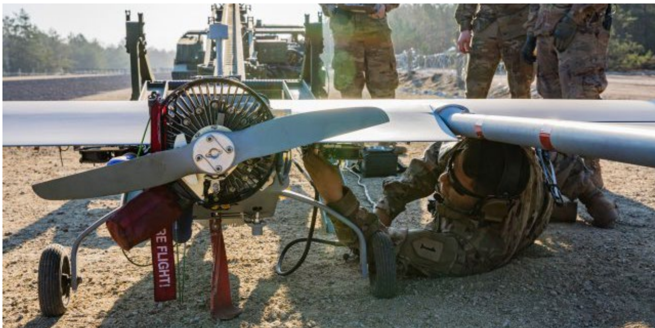
Pfc. Anthony Garcia, an Unmanned Aircraft Systems Repairer with the 1st Eng. Bn., conducts preflight checks on an RQ-7 Shadow Unmanned Aerial Vehicle prior to takeoff during a surveillance training mission at Camp Trzebień, Poland.
