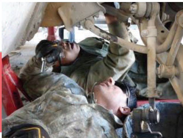
Fredricksburg, Va. native Spc. Melvin Lawson (top of photo), all-wheel vehicle mechanic, Company B, 46th Engineer Combat Battalion (Heavy) shows Spc. Malik, 6th Iraqi Army Division, mechanic, how to install a new radiator hose while underneath the military vehicle, 26 March.
