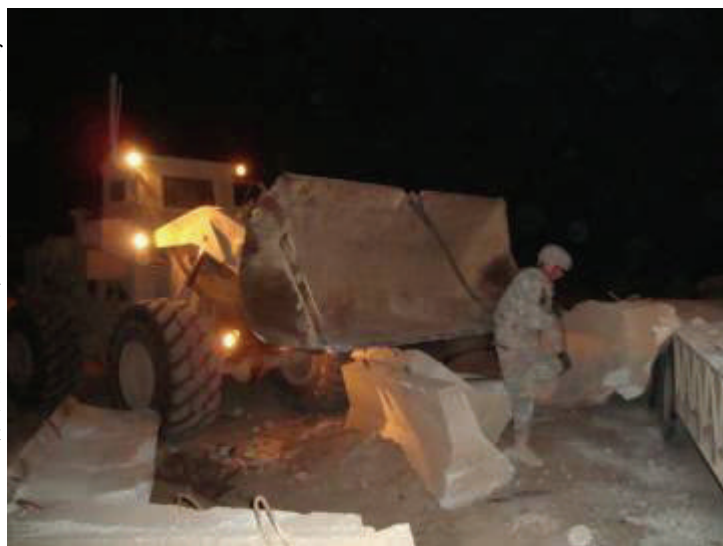
Sgt. Ross Maki, 46th Engineer Combat Battalion (Heavy), 225th Engineer Brigade, 1st Cavalry Division, Multi-National Division - Baghdad, a native of Lake Linden, Mich., utilizes the loader and chains to yank jersey barriers from a trailer for disposal in the barrier yard.
