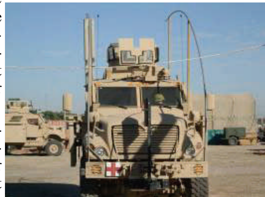
Soldiers conduct a test of the wire mitigation system by passing an mine resistant ambush protected under low-hanging wires.
