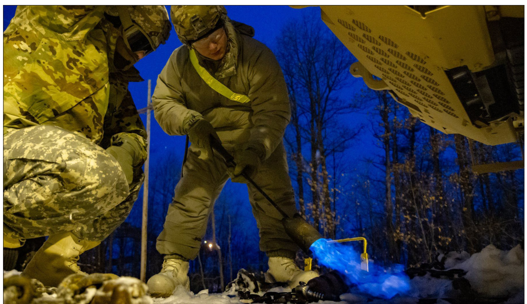
A Soldier from 1st Brigade Combat Team uses a blowtorch to melt heavy ice off tie-down chains to prepare for rail-load operations ahead of their scheduled rotation to JRTC.
