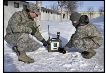
Senior Master Sgt. Amber Westie waves gasoline beneath the sensor of the Area RAE pro, a long range contaminant detection monitor while Tech. Sgt. Marcus Jackson, 120th Airlift Wing readiness and emergency management flight specialist, verifies the alarm was tripped. (U.S. Air National Guard photo/Staff Sgt. Lindsey Soulsby)
