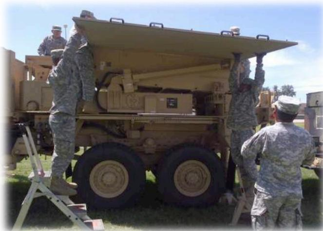
**During the New Equipment Fielding (NET), 1-7 FA BN’s Radar section completed PMCS on the AN/TPQ-53. These pictures depict the radar crew removing the radome cover of the radar. The crews also performed removal and installation procedures on other sections of the radars.**
