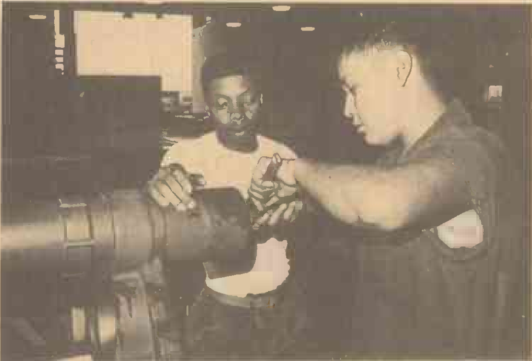
EASY DOES IT — Private First Class Anderson Dyer (right) works on the recoil mechanism of a 105mm howitzer while Sergeant Jermel Johnson observes.
